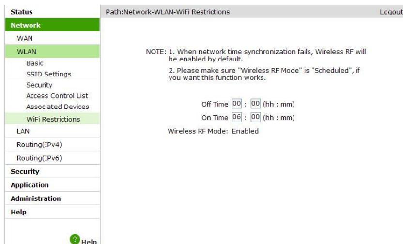
NOTE: 1. When network time synchronization fails, Wireless RF will be enabled by default.
