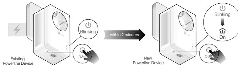
4. When the Powerline LED
