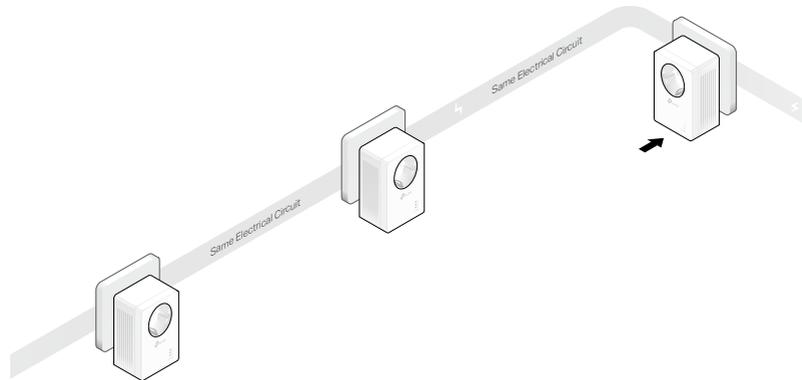
2. Press the Pair button on any of the existing powerline devices for 1 second. Its Power LED
